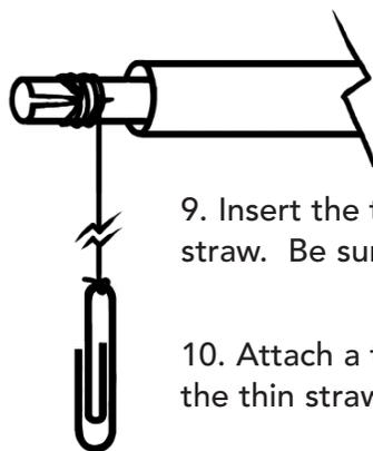
9. Insert the thin straw into the large straw. Be sure it turns freely
