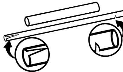
4. Cut slits at the ends of the thin straw.
